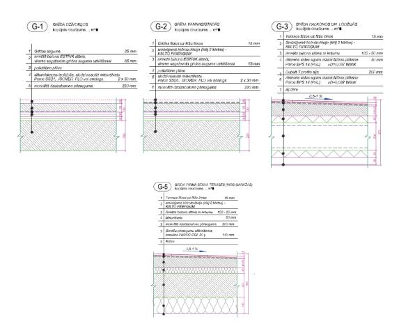
Roof construction: operated, flat, and for apartments on the upper floors with entrance to the terrace.
